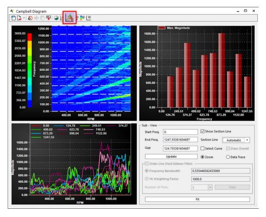
• Overall Curve: In the Slice View of the Campbell diagram for RPM-Order, it is now possible to draw an Overall Curve that sums up all the graphs for each frequency.
