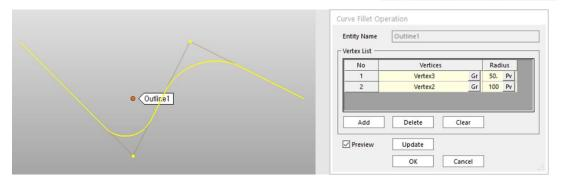
Midpoint of Outline/Spline: It is now possible to insert Midpoints to the segments of existing Outlines and Splines. In addition, a Preview function for each point, and a function to adjust the first Derivative of the Spline have been added. The use of Midpoints is efficient since the added points can increase the curve's precision.
